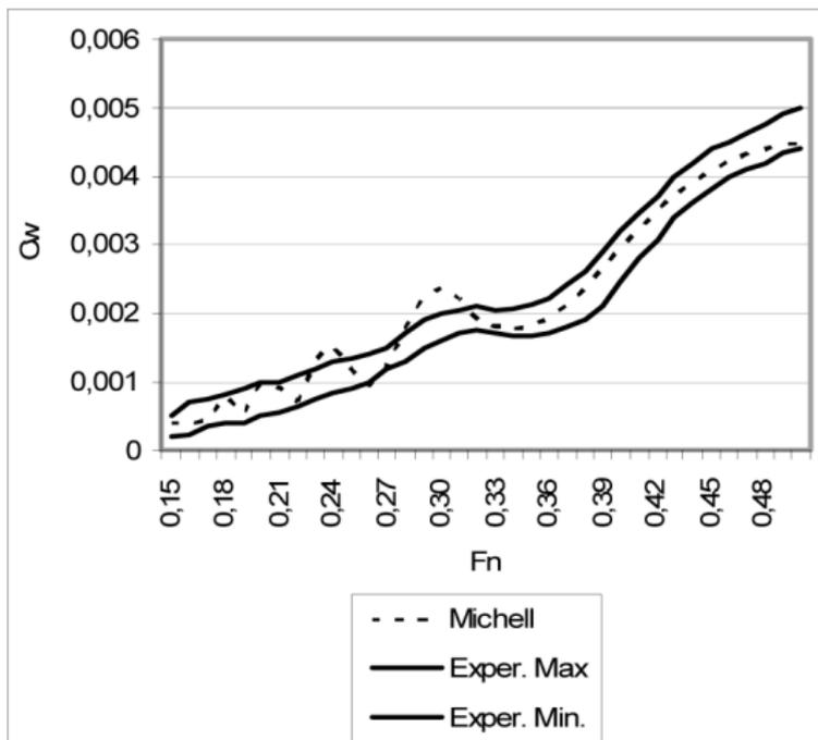
Comparison Michell and experimental data (parabolic Wigley model, **Bai'79**)
