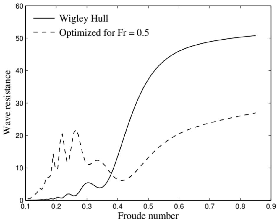
Optimized hull vs. Wigley hull
