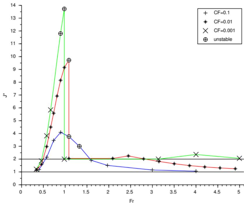
Figure:  $J_{num}^*$  vs  $Fr_a$  for three different drag coefficients
