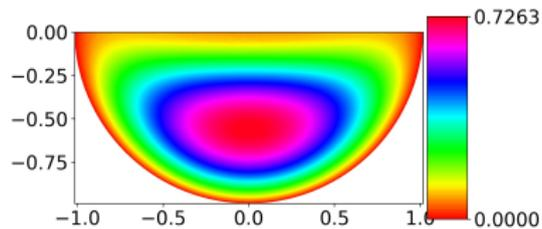
Optimal hull based on a half-disc for  $Fr_a = 1.75$
