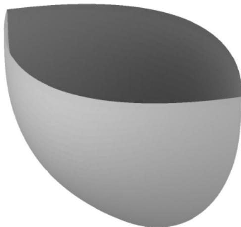
Figure: Optimal hull for  $Fr_a = 4.90$
