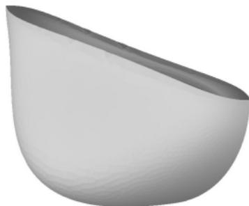
Figure: Optimal hull based on a half-disc for  $Fr_a = 1.75$
