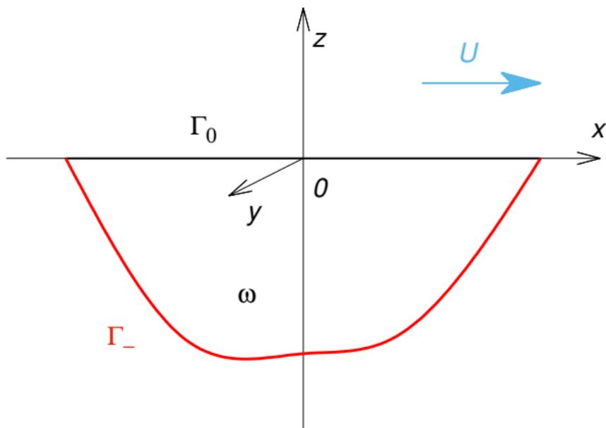
Consider a ship moving with constant velocity  $U$  on the surface of an unbounded fluid.
